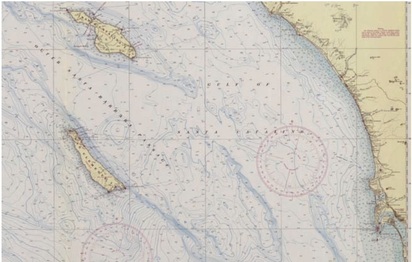
FIG. 386. DETAIL FROM U.S. COAST AND GEODETIC SURVEY CHART, SAN DIEGO TO SANTA ROSA ISLAND, 1939. This prototype chart (5101A) was based on data acquired through RAR (radio acoustic ranging) surveys.
