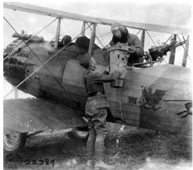
FIG. 1073. WORLD WAR I AIRCRAFT WITH EARLY MAPPING CAMERA. Observer receiving French camera with Berthiot color lens for reconnaissance and photo work, Gondreville-sur-Moselle, France, 6 August 1918. Image courtesy of the U.S. National Archives, Washington, D.C.
