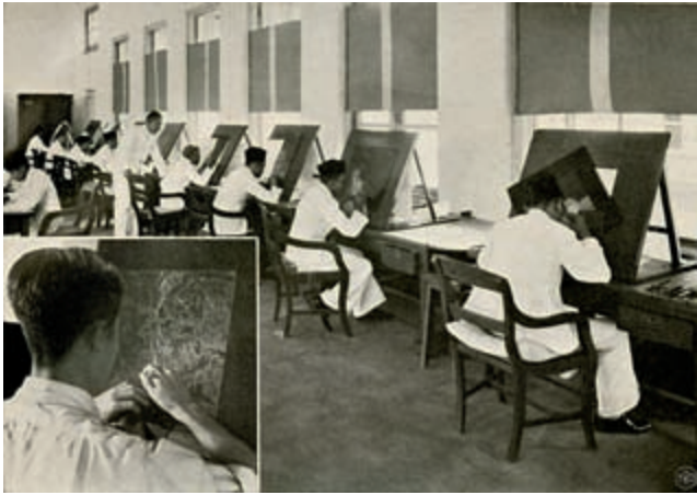
FIG. 889. TOPOGRAPHIC MAP PRODUCTION BY SCRIBING ON GLASS AT THE TOPOGRAFISCHE DIENST OF BATAVIA, 1927.
