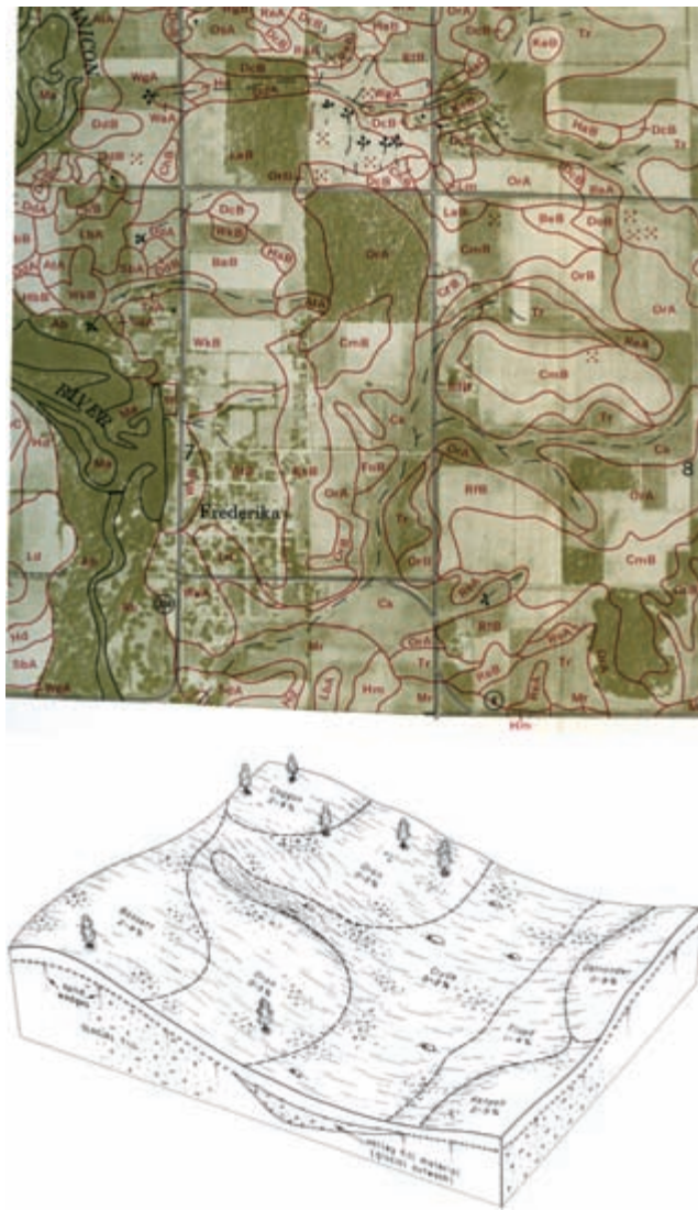
FIG. 910. SOIL SURVEY MAP AND ASSOCIATION DIAGRAM, BREMER COUNTY, IOWA. Bassett (Be), Clyde (Ck), and Oran (Or) soils comprise about 60 percent of the association around Frederika. For areas that are not level or nearly level, a capital letter (A through F, least to greatest) indicates the slope. The relationship of slope, vegetation, and parent material is shown in the association diagram. Size of the entire original (top): 26.6 × 39.5 cm; size of detail: 14.4 × 13.9 cm; size of the original (bottom): 12.3 × 18.8 cm. From Soil Survey: Bremer County, Iowa ([Washington, D.C.]: U.S. Soil Conservation Service, 1967), sheet no. 13 and p. 4 (fig. 3).
