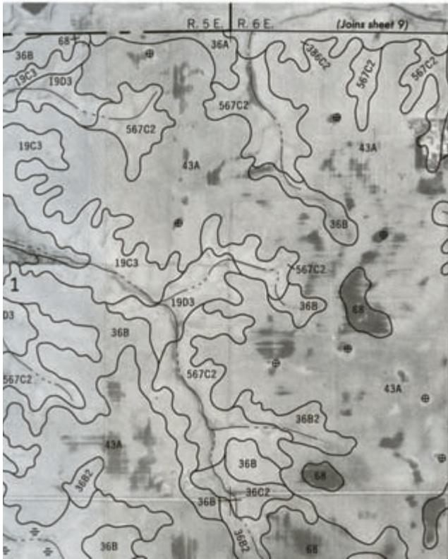
FIG. 909. DETAIL FROM COUNTY SOIL SURVEY, STARK COUNTY, ILLINOIS. Poorly drained soil (dark color) and well-drained soil (light color) are visually quite distinct in this part of the United States, but it is also clear that soil surveyors have to make judgments in order to map soils at the desired level of generalization. As a result each delimited area tends to include smaller areas of different soil.
