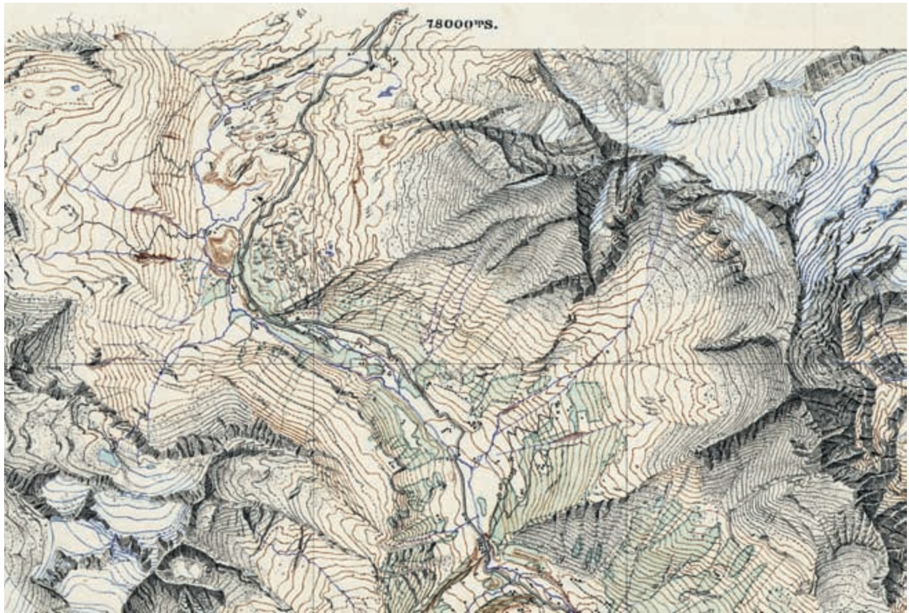
FIG. 213. DETAIL FROM PLANE TABLE SURVEY SHEET SIMPLON (SHEET 501), 1886/87. Multicolored manuscript drawing at the original scale of 1:50,000 by Xaver Imfeld for the national topographic map series of Switzerland (called the Siegfriedkarte). The extract depicts the Fletschhorn and the
