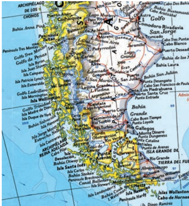
FIG. 168. DETAIL FROM SOUTH AMERICA, BY JOHN F. SHUPE, 1:11,890,000. This example of a highly developed printing practice employed yellow, cyan, magenta, black, a special blue, and grayish brown inks printed, singly or in combination, solid or screened, to create the various outlines of the countries, relief, line symbols, and lettering with precision and clarity.
