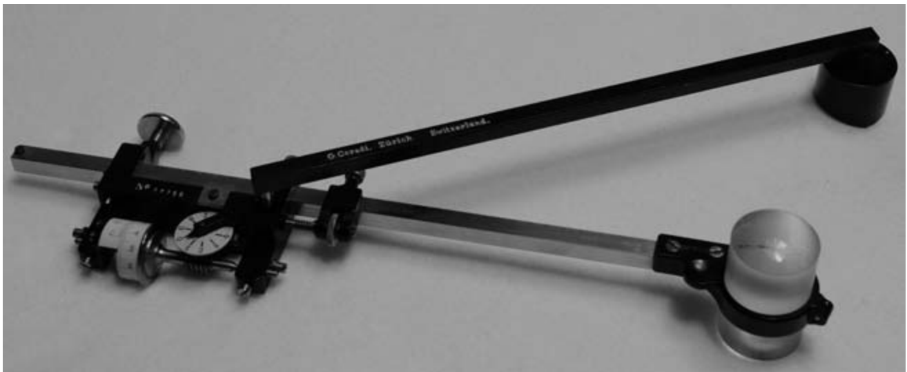
FIG. 127. POLAR PLANIMETER, MADE BY G. CORADI, ZURICH, CA. 1937. The circular weight to the upper right is static while the user traces the figure with the circular magnified cursor, accumulating the area on the scale on the "elbow" via a roller in contact with the surface.
