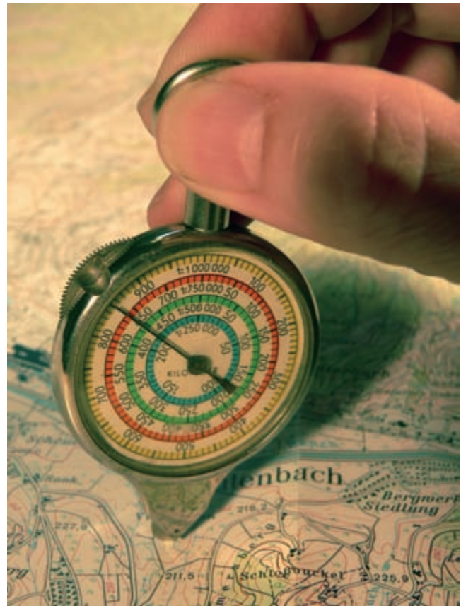
FIG. 129. AN OPISOMETER, ALSO CALLED A MEILOGRAPH OR MAP MEASURER. The instrument is used for measuring the lengths of arbitrary curved lines. Image courtesy of Frank C. Müller.
