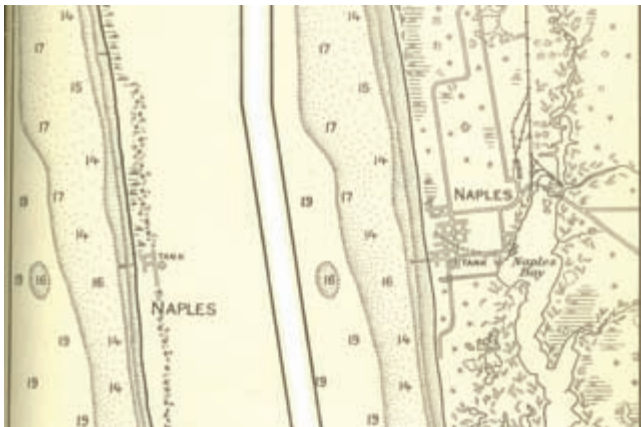
FIG. 155. COASTAL CHART COMPARISON. Corresponding portions of a coastal chart for an area near Naples, Florida, using a limited ground survey (left) and aerial photography (right).
