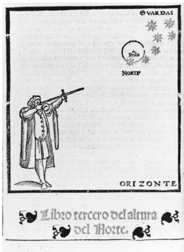
FIG. 20.8. ILLUSTRATION OF A MAN MEASURING A STELLAR ALTITUDE USING A CROSS STAFF.
