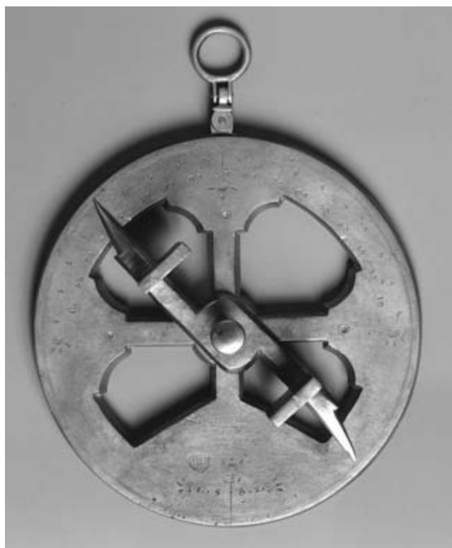
FIG. 20.5. A TYPICAL MARINER'S ASTROLABE, OF SPANISH MANUFACTURE, 1563. This modest instrument is scaled down from its astronomical cousin.
