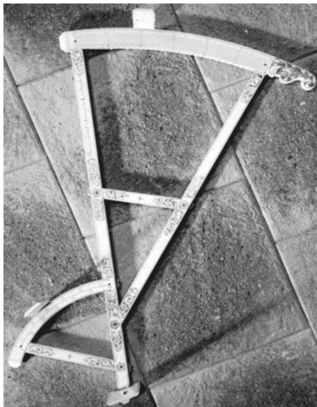
FIG. 20.9. AN IVORY BACK STAFF, ENGLISH, 1690. Typical of seventeenth-century models. Made by Thomas Tuttell. Photograph © National Maritime Museum, London (neg. no. D4504).
