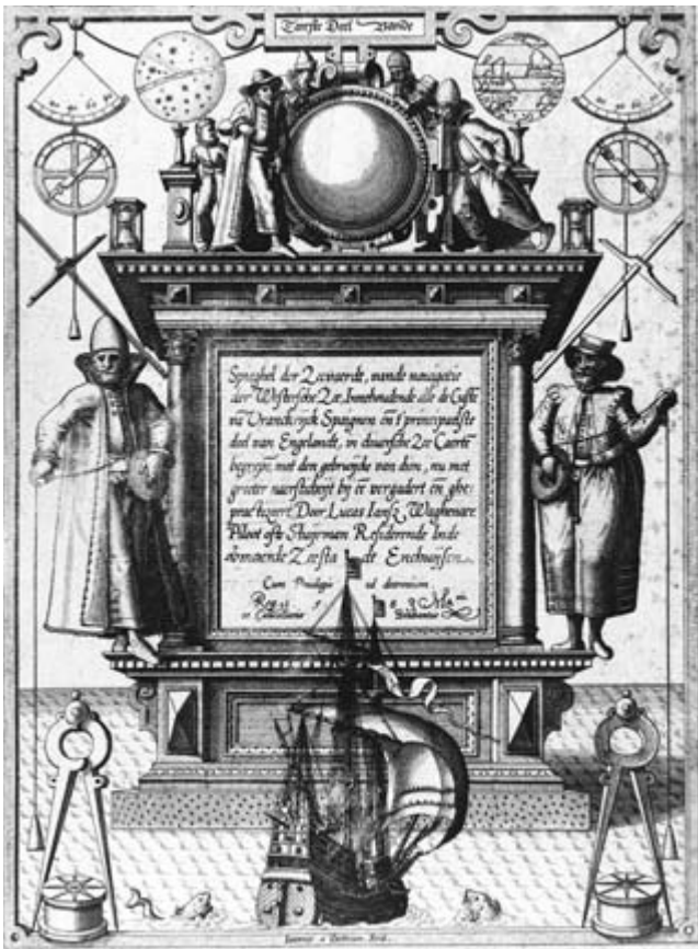
FIG. 20.3. THE TITLE PAGE FROM WAGHENAER'S SPIEGHEL DER ZEEVAERDT , 1584–85. The frontispiece depicts a number of common early modern navigational instruments, including the quadrant, astrolabe, cross staff, dividers, and box compass, all of which are depicted, respectively, from top to bottom along each side. Each of the male figures (on either side of the title itself) is holding a lead and line. Size of the original: 37 × 24 cm. Lucas Jansz. Waghenaer, Spiegel der zeevaerdt (Leiden: Christoffel Plantijn, 1584–85). Photograph courtesy of the James Ford Bell Library, University of Minnesota, Minneapolis.
